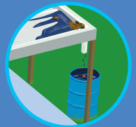
Flat roof without adequate drainage
