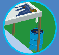
Flat roof without adequate drainage
