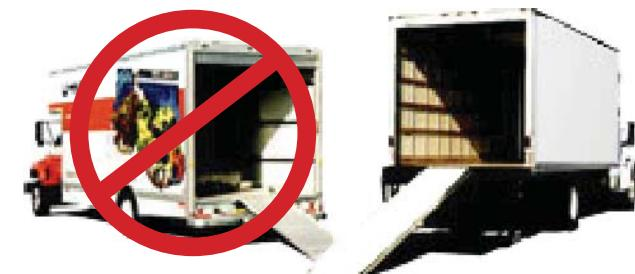
In the above photo the trucks are both 24-foot trucks, however the truck on the left could not be loaded from a RSS or RDS loading dock. There is a 16-inch difference between the height of the truck and the loading dock.
