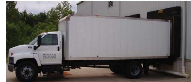
The above truck is an example of a 20 foot truck which has a bed height of 48 inches and meets level with the loading dock.
