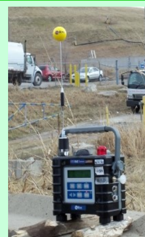
Missouri Department of Natural Resources used an AreaRAE® multi-sensor system to test air for various chemicals including sulfur-based compounds.
