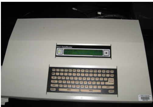
An example of a BAC DataMaster which is an infrared electronic breath alcohol measuring instrument.
