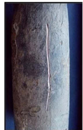
Picture of a Scratch on a Lead Service Line
