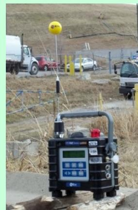
Missouri Department of Natural Resources used an AreaRAE® multi-sensor system to test air for various chemicals including sulfur-based compounds.
